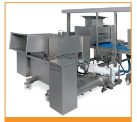
The Rijkaart fat/butter pump especially developed to sheet all types of fat, margarine and butter from a block into a continuous band. The width and thickness of the fat sheet can be accurately adjusted in a matter of seconds simply by changing the front plate of the fat nozzle.
