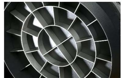
Anodized coated aluminium dividing disc and stainless steel knife require minimal flour for dividing and are hygienic in use.
