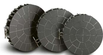
On the Variomatic product quality is increased by additional parameters matching dividing discs with dough type: rounding speed and rounding stroke. The weight setting is programmable through the control panel.
