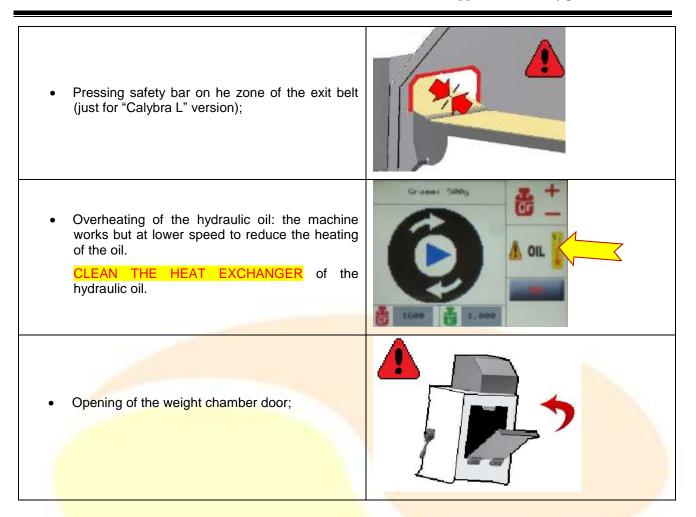
To restart the work after emergency stopping, it is necessary re-establish the beginning situation, so:
