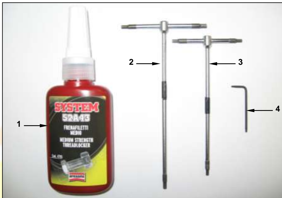
Figure 35 – Equipment for disassembly/assembly of micro switches associated with the sensor ring
