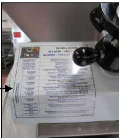
Figure 40 - Machines with electro-mechanical panel: adhesive with legend of alarm signal lights
