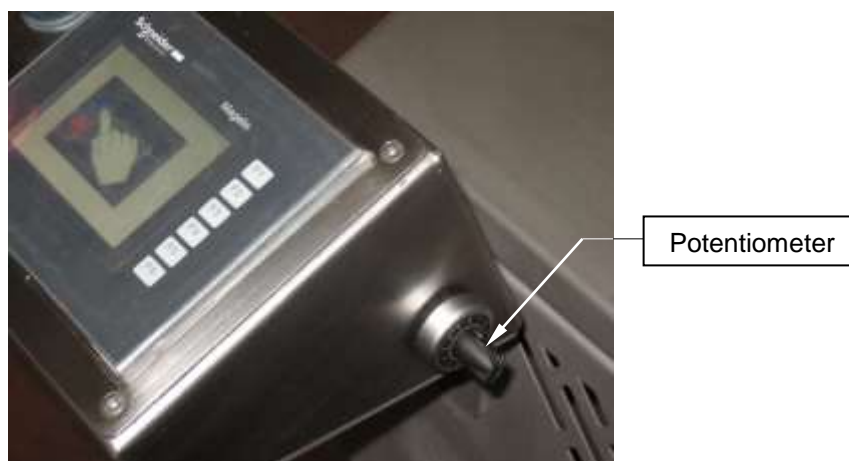
Figure 9 - «V»-belt relative speed potentiometer
