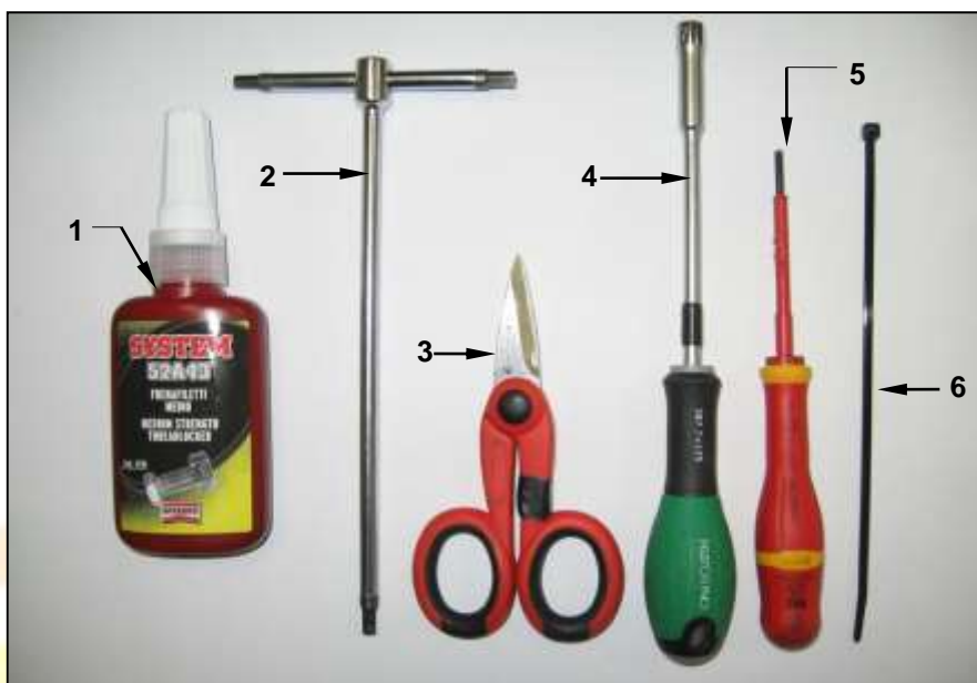
Figure 38 – Equipment for replacing the micro-switch associated with the weight chamber door
