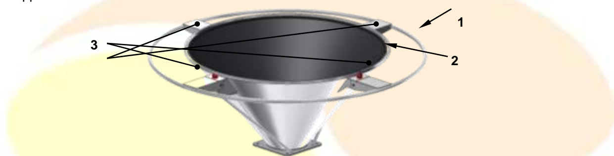
Figure 29 – Sensor ring and spacer ring of the hopper
