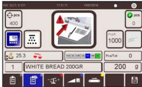
After loading the recipe, if the recipe requires single or splitted division, requiring manual setting of the single or double selection lever, the adjacent screen is displayed: the machine can only be started after the mobile handle has been rotated correctly.
