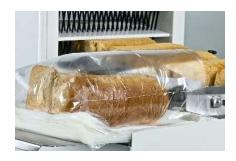
After slicing of the bread, a bag blowing device automatically opens the plastic bag. Sliced bread is inserted manually in one natural movement, saving considerable time.
