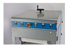
Independently variable speed for inand outfeed belt, reverse button for last bread, height-adjustable upper infeed conveyer belt.
