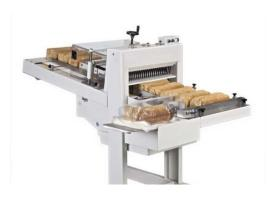
Double in-feed belts with electronic variable speed.
