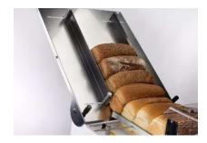
Optional chute for extra bread infeed storage for up to 15 breads. Chute with side guide strips for different seizes of bread and can be folded down completely when not in use.
