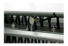
Optional automatic oil lubrication system prevent sticking of crumbs on blades. In particular recommended for slicing darker bread types.
