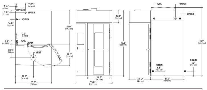
Highest Point on Oven: 104" (265cm) Rack Swing Diameter: 34.5" (87.6 cm) KD Shipping Weight: 2,580 lbs. (1170kg) (shipped whole)/3,070 lbs. (1393kg) (shipped split)
